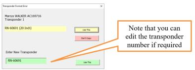
Where the auto-correction is not possible, the operator can enter the valid transponder number in the green box then click the corresponding "Use This" button.
